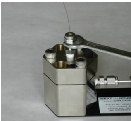
Figure 6. Use a wrench to tighten the nut, forcing the ferrule to squeeze tightly around the capillary.
