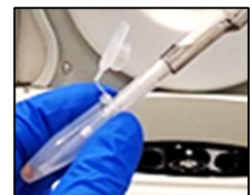
Figure 5: Using the tip of a pipette, carefully remove all of the remaining Wash Buffer that has collected just below the magnetic bead pellet.
